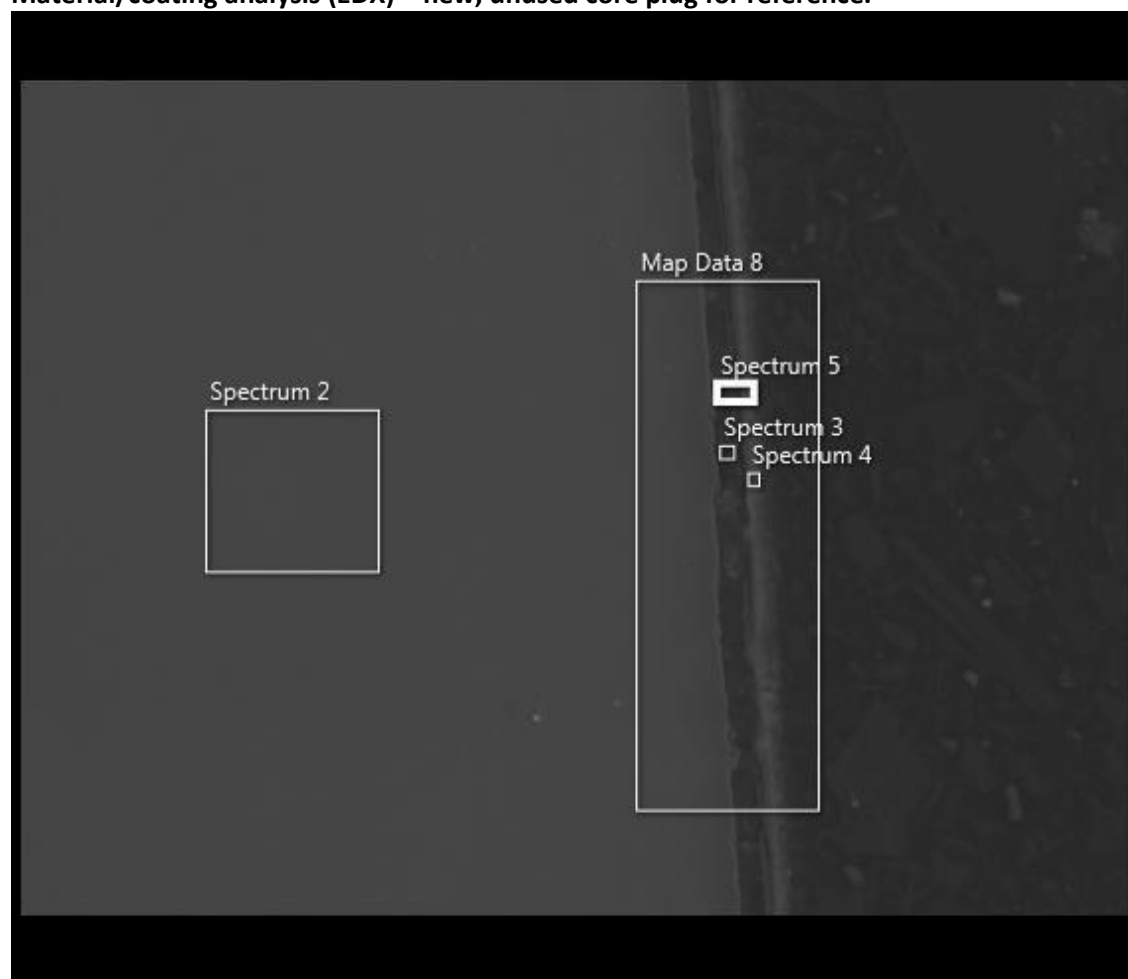
Figure 12: Cross section of new, unused core plug magnified 4,000x.
