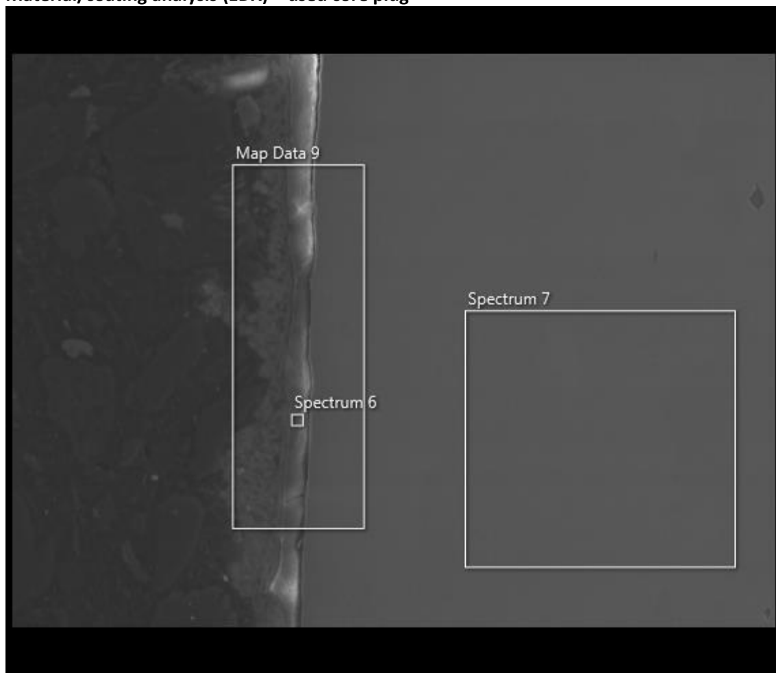
Figure 9: Cross section of used core plug magnified 4,000x.
