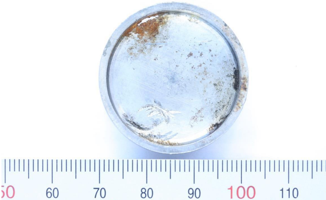
Figure 8: Outside, 1 little core plug from rear cylinder head after cleaning with acetone and ultrasound.
