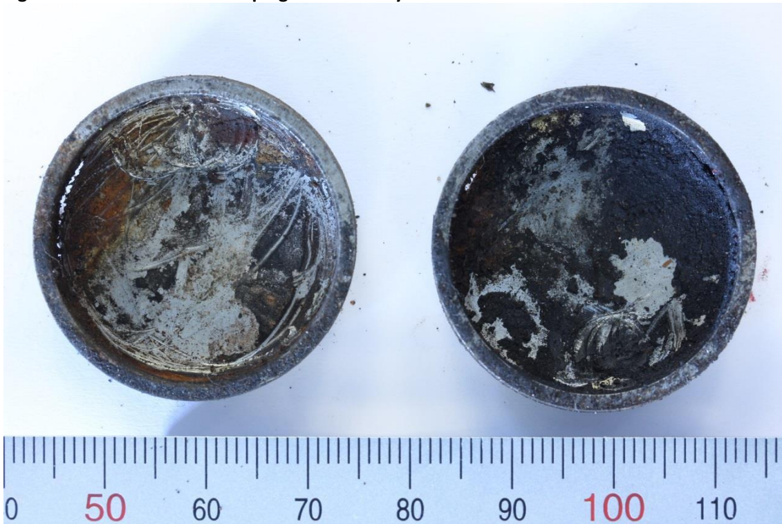
Figure 6: Outside, 2 small core plugs from rear cylinder head.
