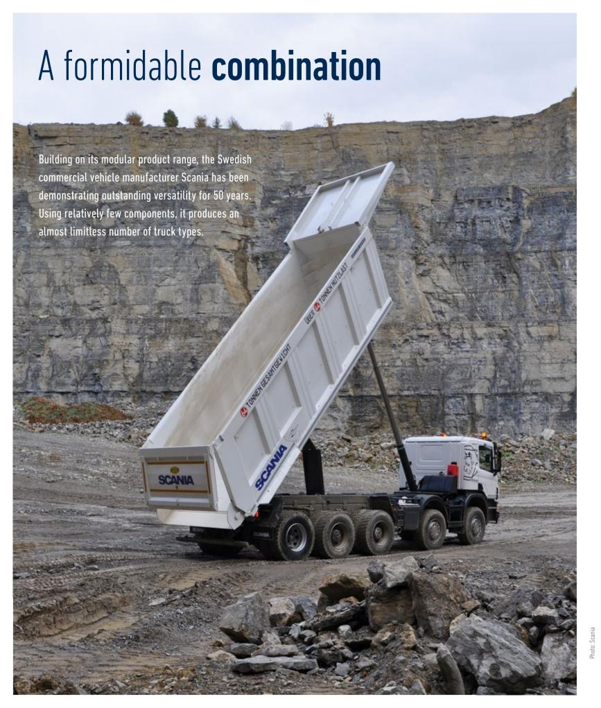
cania can supply a rugged standard truck for the majority of demanding transport tasks. If the load and laden weight requirements are exceptionally high, however, it turns to BPW to enhance its vehicles' capabilities with a steered tag axle. These axles are typically installed behind Scania's own drive axles, but they are also to be found in the heavy trucks that operate in coal, ore and gold mines, as well as in quarries.
